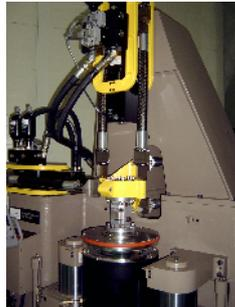
Fig. 8. Bushing test using MTS 3-axes tester.
